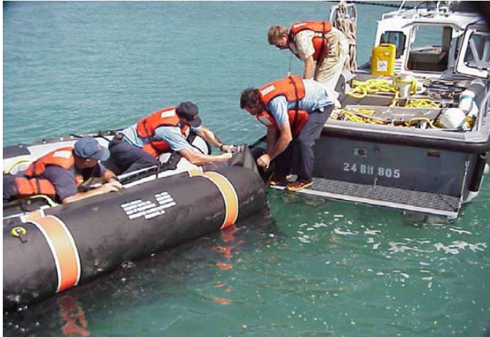
Open Ocean Containment Boom Deployment
