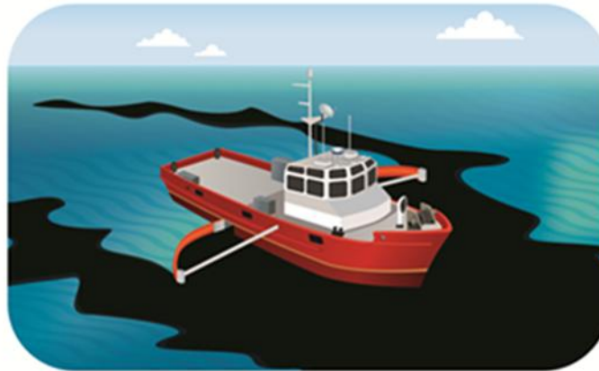
Mechanical Containment & Recovery
